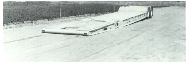
Lowbed semi-trailer with hydraulically controlled gooseneck in lowered position for loading.
