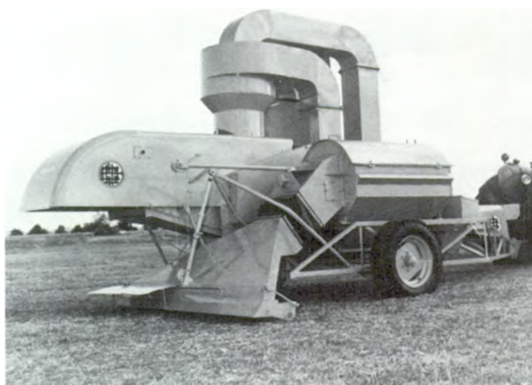
Towed vacuum-operated seed harvester.
