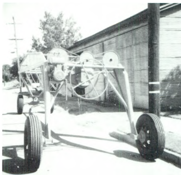
Straddle-type implement carrier.
