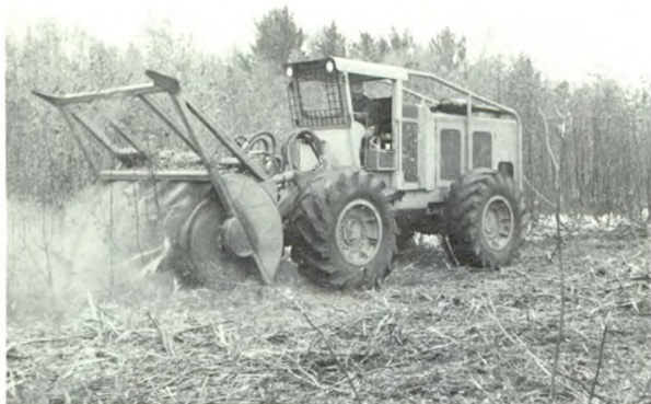
Self-propelled rotoheater shredder masticating brush.
