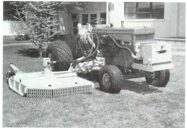
Hydraulically powered rotary cutter.
