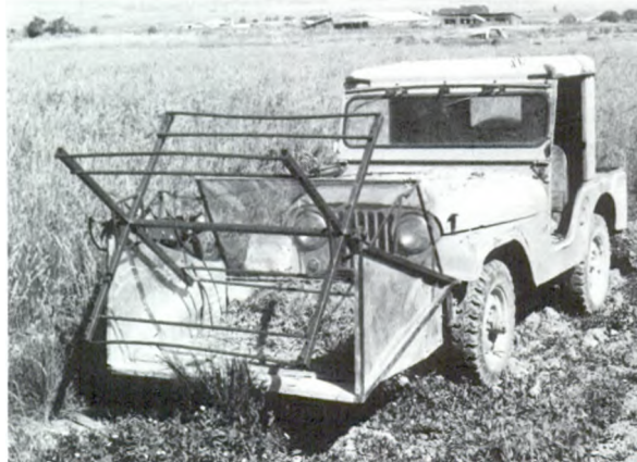
Grass stripper reel mounted on a jeep.
