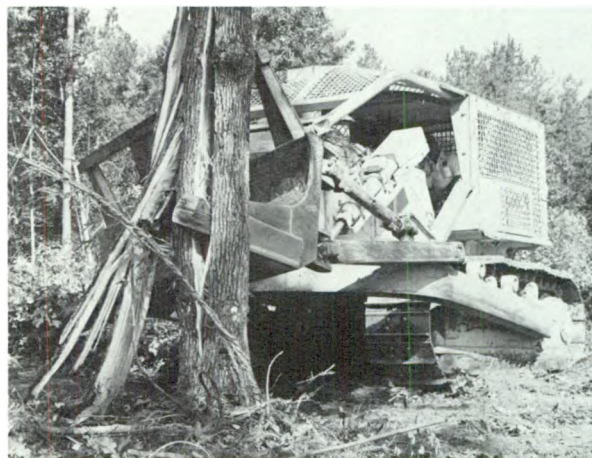
Shearing blade clearing trees.
