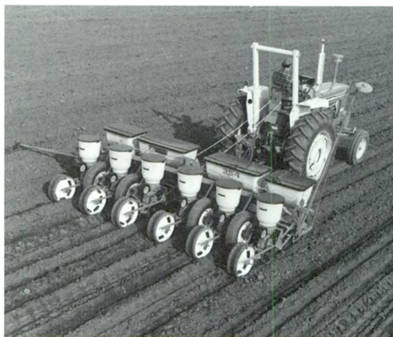
Air-powered planter units on a frame.
