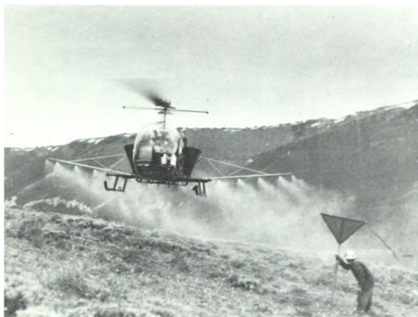
Helicopter boom sprayer with side tanks.
