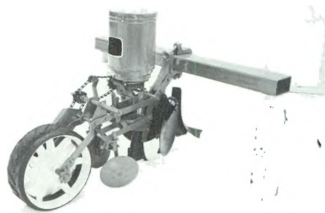
Standard unit planter on a toolbar.
