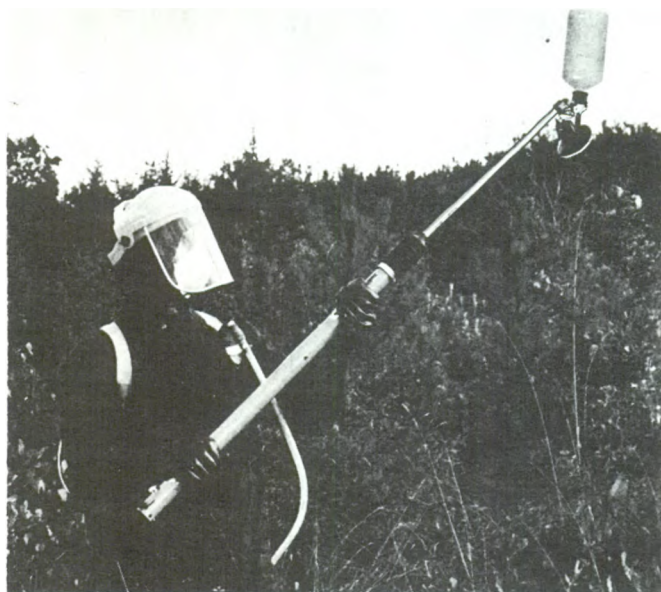
Low-volume applicator for treating large areas by hand.
