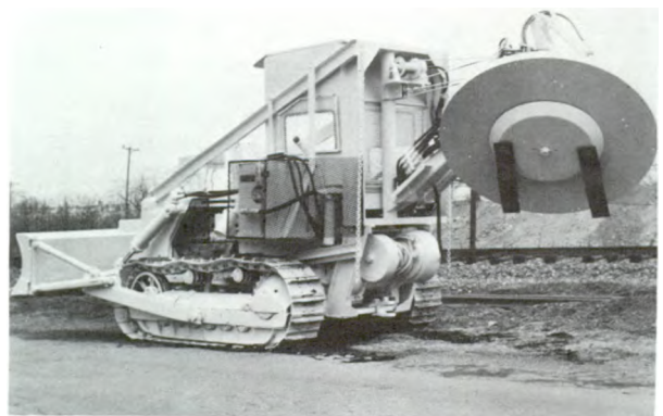
Boom-mounted rotary cutter.
