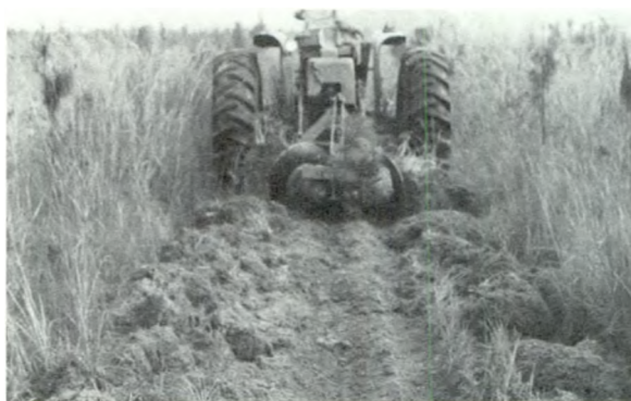
Fireplow cutting a wide, shallow furrow.
