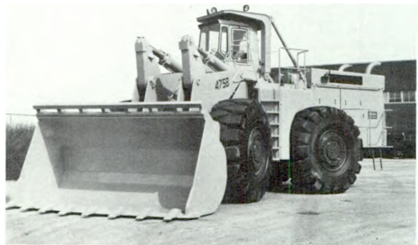
Large articulated front-end loader commonly available at mine sites.
