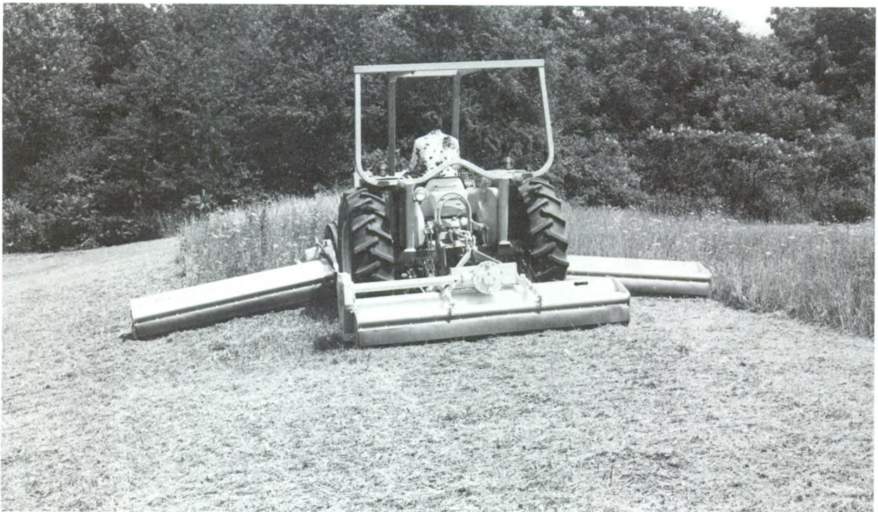
Three gangs of rotobeater mowers featuring both hydraulic and power-take-off drive.
