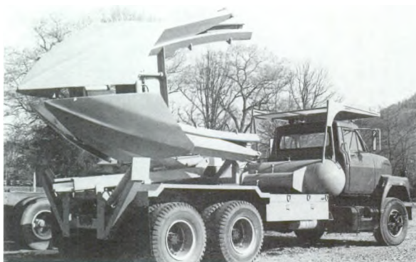
Large tree spade mounted on a truck.
