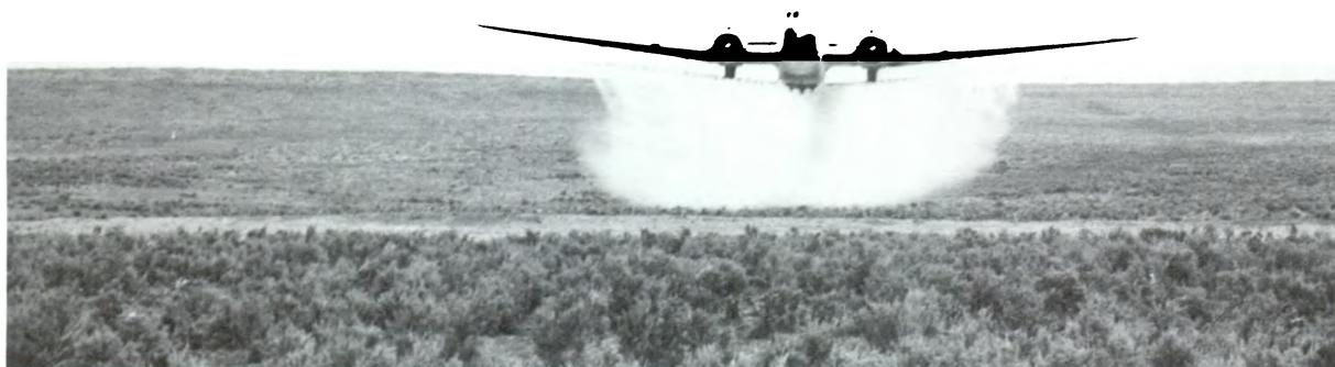
Fixed-wing aircraft sprayer.
