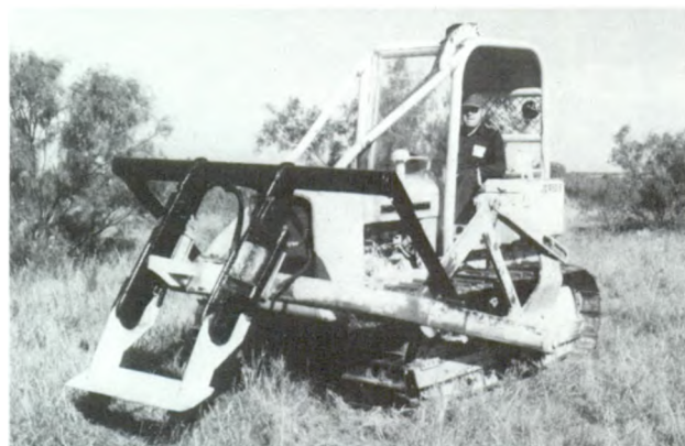
Hydraulic grubber mounted on a C-frame.
