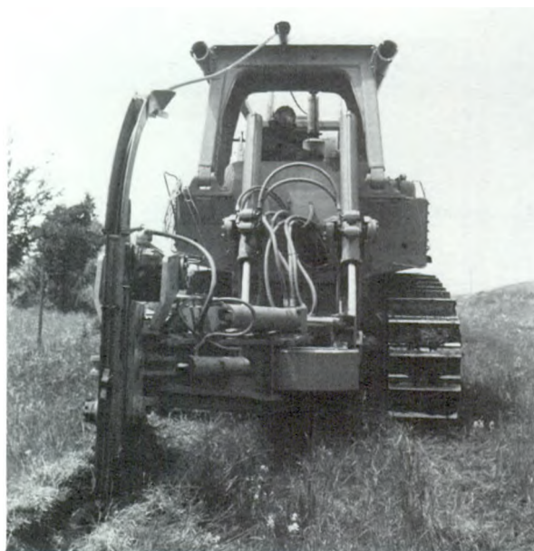
Cable plow with full hydraulic control.
