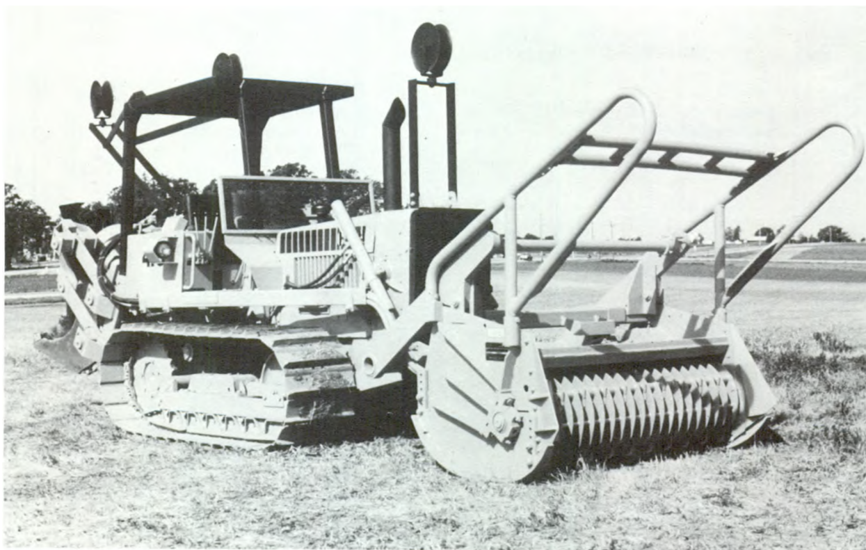
Rotobearer shredder mounted on a crawler-tractor.
