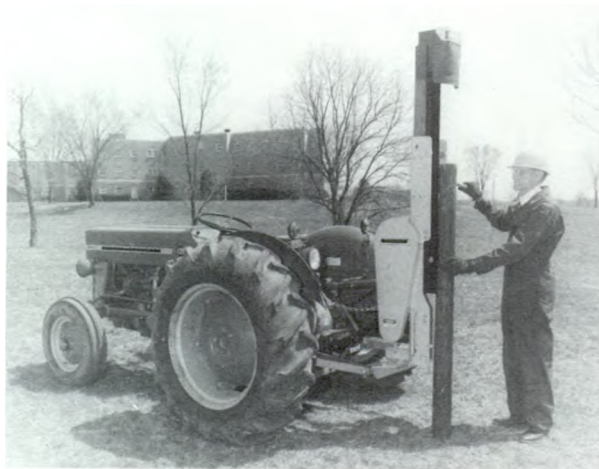
Power-take-off post driver mounted on a three-point hitch.
