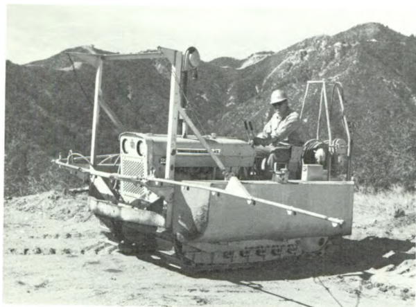
Side-mounted spray tanks on a small crawler tractor.
