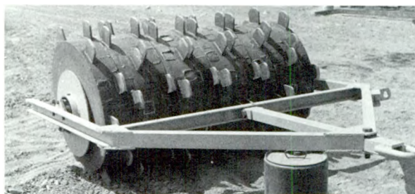
Flexible cultipacker with large steel rings.
