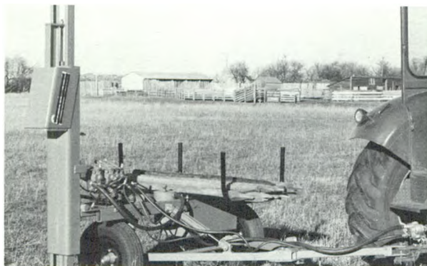
Post driver mounted on a separate trailer.
