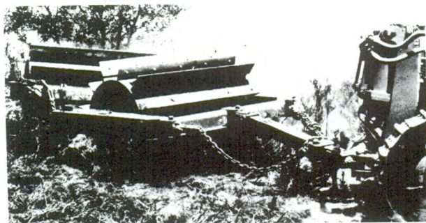
Tandem rolling choppers towed in an offset configuration.
