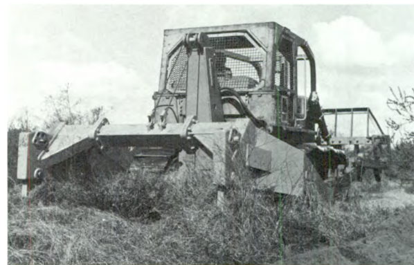
Root plow controlling brush by slicing roots.
