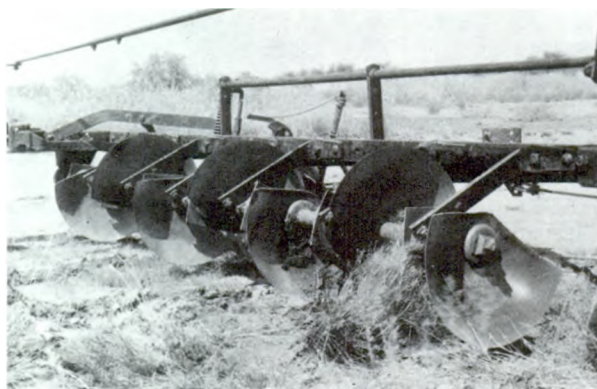
Cuttout disks on a pitting disk plow.
