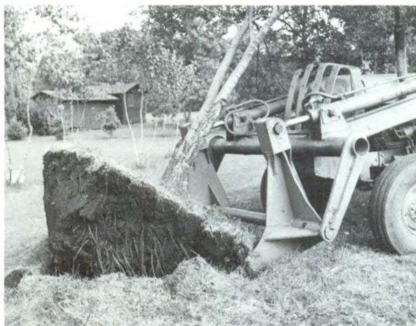
Single blade transplanter removing a small tree.
