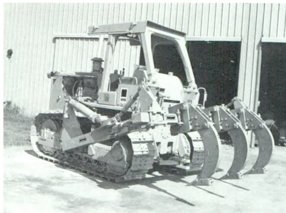
Subsoilers attached to a crawler tractor toolbar.
