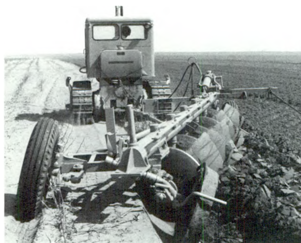
Large one-way disk plow with separate disks.
