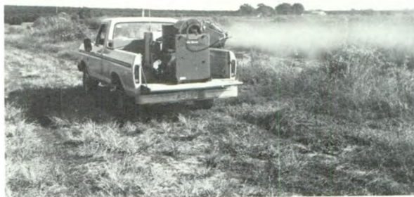
Truck-mounted mist sprayer for controlling brush. (Automatic Equipment Mfg. Co. photo)
