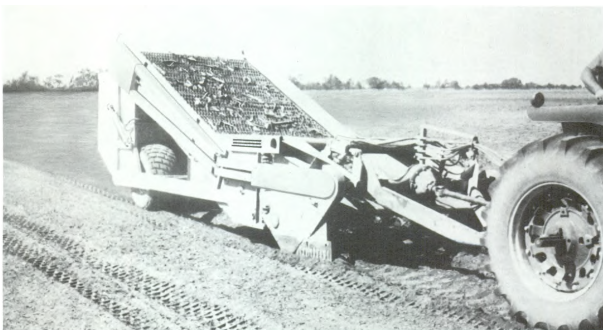
Soil sifter with chain conveyor.
