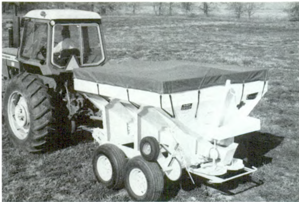
Trailer-mounted fertilizer spreader with a wheel-driven belt.
