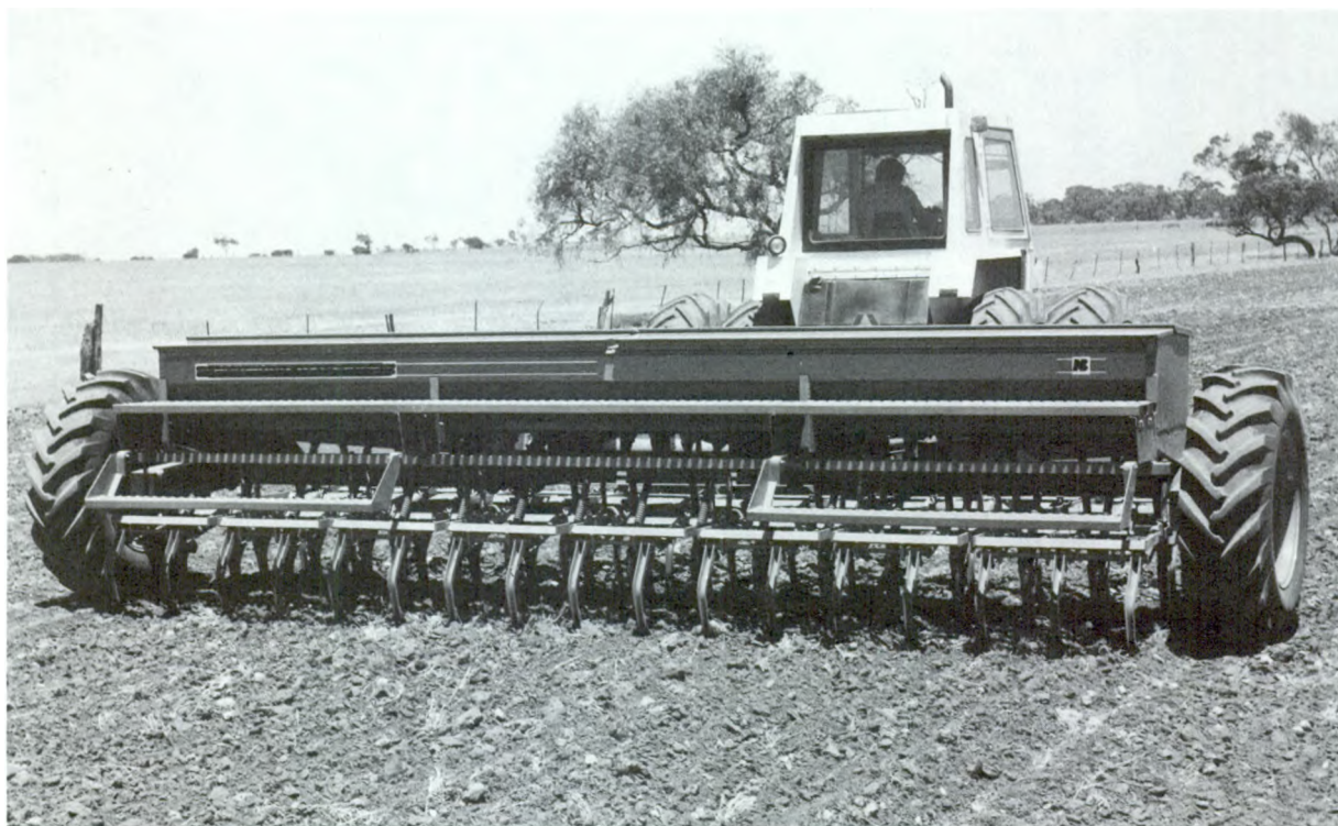
Grass drill with chisel openers.
