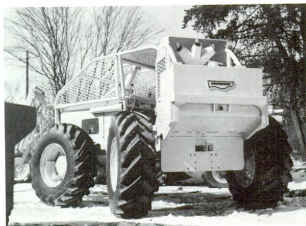
Mist sprayer on a logging skidder.
