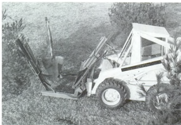
Three-blade tree spade with open digging platform.
