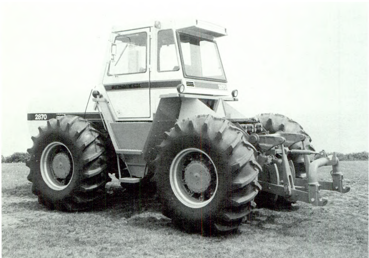
All-wheel drive tractor with independent steering of front and rear wheels.
