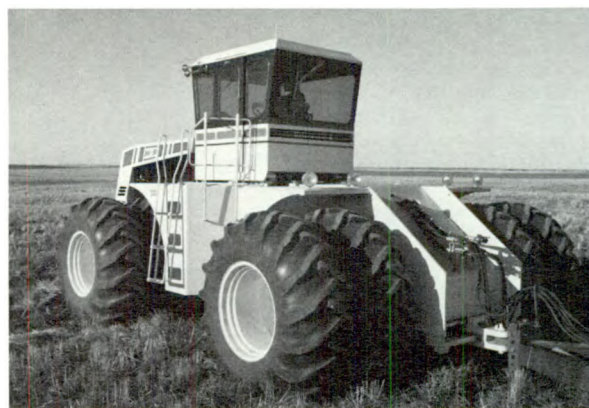
All-wheel drive tractor with articulated steering.
