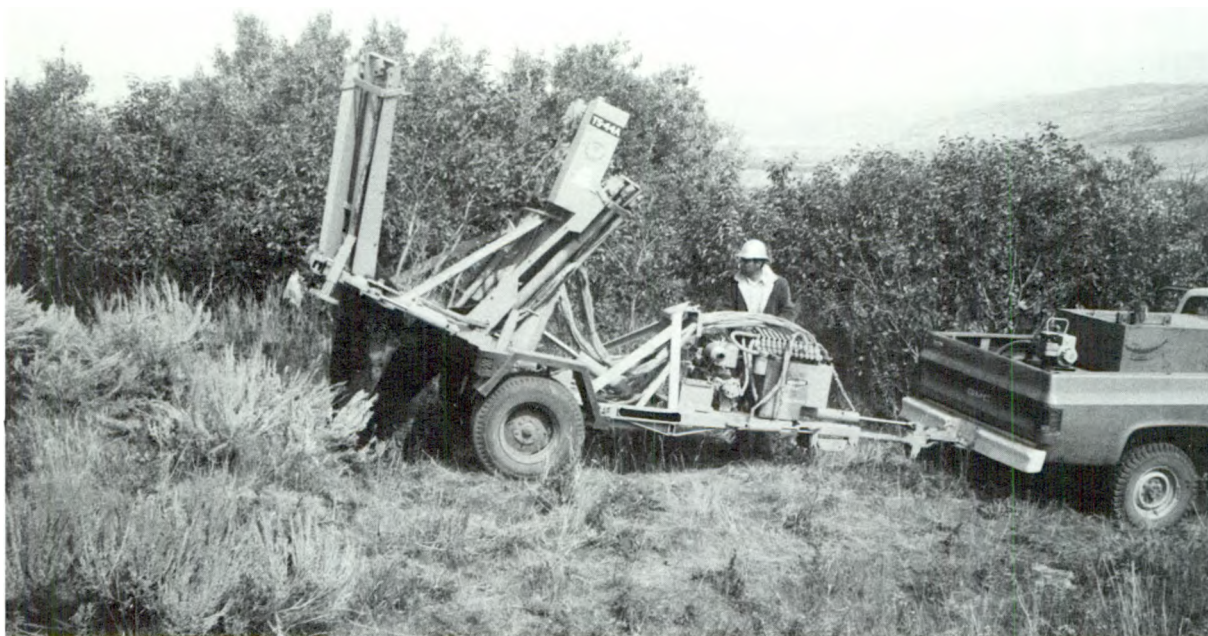
Trailer-mounted four-blade tree spade.
