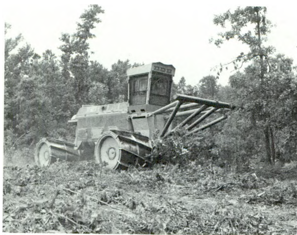
Large self-propelled rolling chopper.
