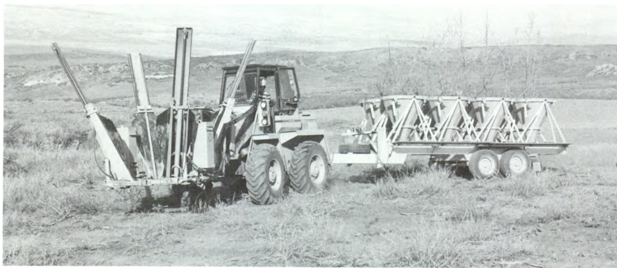
Tree transport trailer towed by a small front-end loader equipped with a tree spade.
