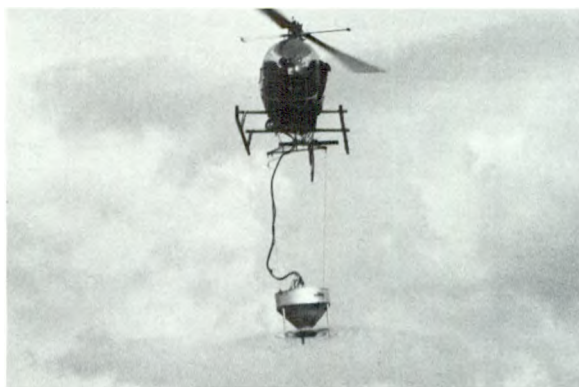
Rotary spreader suspended beneath a helicopter.
