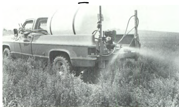
Skid-mounted broadjet sprayer.
