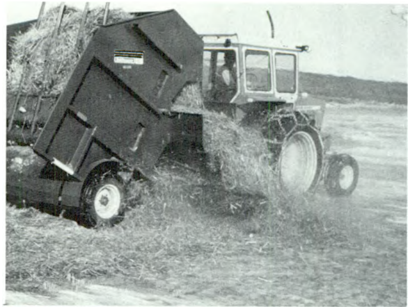
Hesston stakprocessor with MacFarlane flail to distribute straw mulch from round bales.
