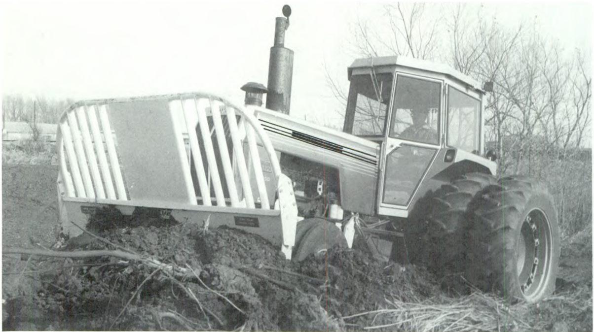
Three-way dozer on a rubber-tired tractor.
