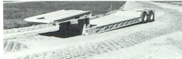
Lowbed semi-trailer with hydraulic gooseneck raised for transport.
