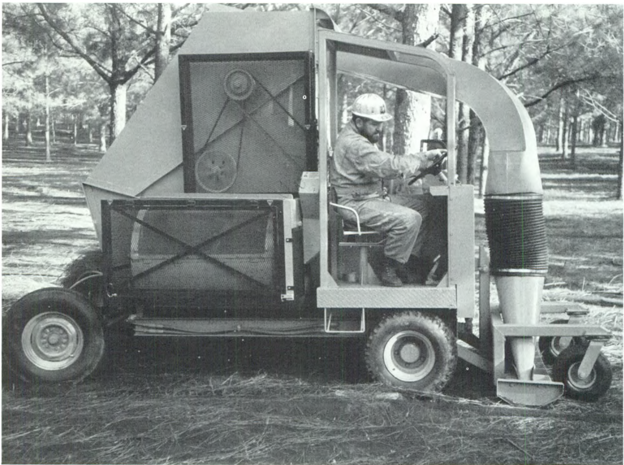
Self-powered vacuum seed harvester.
