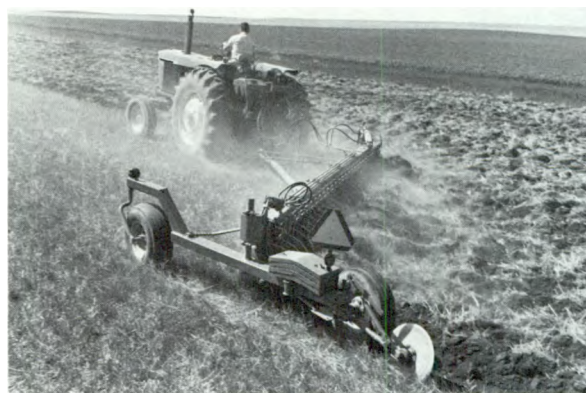
One-way tiller disk plow.
