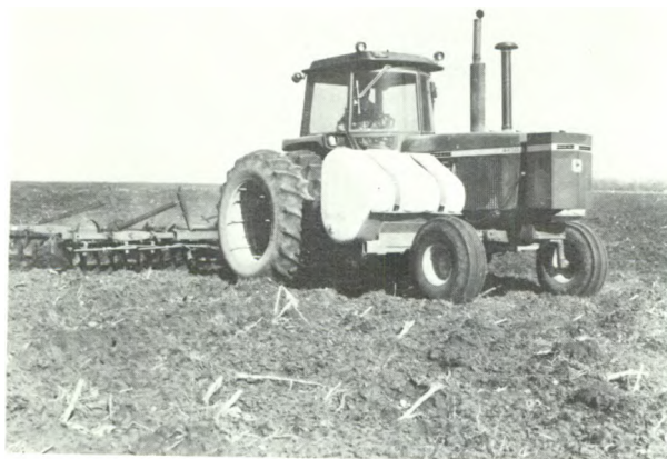
Side-mounted tanks for spraying in front of tillage implements.
