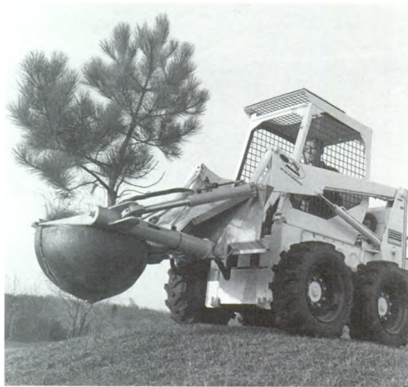
Three-blade tree spade on a skid-steer loader.
