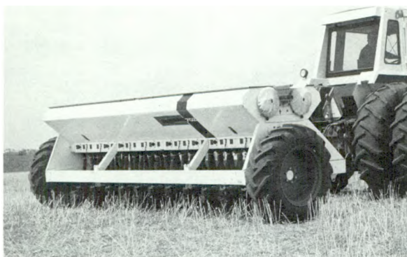
Pasture drill with double-disk openers and coulter disks.
